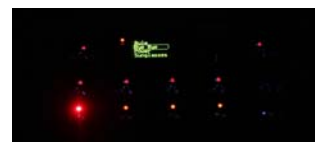
Dimmable LEDs and a high-contrast display enable use on a completely dark stage
