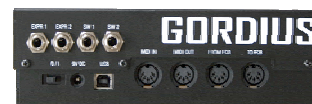
... with extended connectivity : USB, extra MIDI IN/OUT ports, 2 extra external expr.pedals, 2 extra external switches
