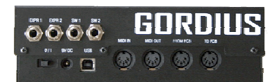
USB, 2 x MIDI IN and OUT, phantom power, 4 jacks for expression pedals or switches
